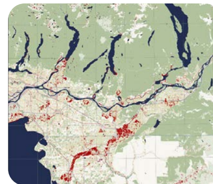
Rapid flood mapping generated with the FloodML algorithm from Sentinel-1 radar images for a flood event over Seattle (US) and Vancouver (CA) on 16/11/2021. © CNES-CLS
